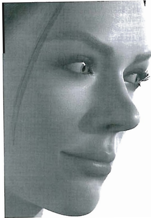
FIGURE A.3.2 GPU-rendered image. To give the skin visual depth and translucency, the pixel shader program models three separate skin layers, each with unique subsurface scattering behavior. It executes 1400 instructions to render the red, green, blue, and alpha color components of each skin pixel fragment.
