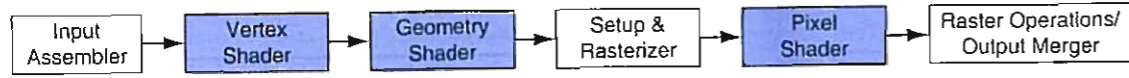
FIGURE A.2.3 Graphics logical pipeline. Programmable graphics shader stages are blue, and fixed-function blocks are white.
