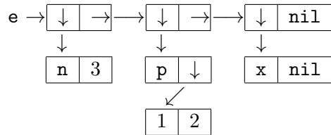
Note that a `CONS` index points to two cells on the stack, the `car` and `cdr` cells.
