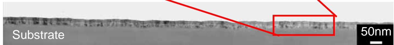
Cross sectional view shows seedlayer, underlayer, intermediate layer, first magnetic layer, interlayer and second magnetic layer. Full thickness of all layers together ~50 nm.
