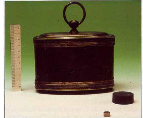
250 years of progress in magnet technology - the lodestone, ferrite and Nd-Fe-B magnets each produce half a Joule of magnetic energy, yet the size of the magnet has decreased a thousandfold. (Photo: Coey, Trinity College Dublin.)
