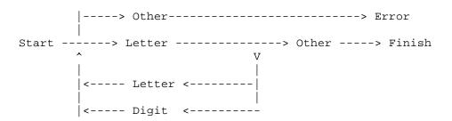
As you can see, this diagram shows how the logic flows as characters are read. Things begin, of course, in the start state, and end when a character other than an alphanumeric is found. If the first character is not alpha, an error occurs. Otherwise the machine will continue looping until the terminating delimiter is found.
